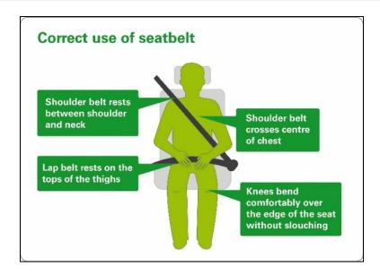
Figure 4 - Correct use of seatbelt
