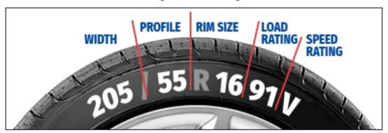
Figure 2 - Tyre markings explained
